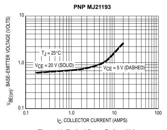
Figure 11. Typical Base-Emitter Voltage
