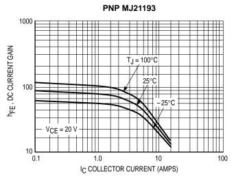
Figure 3. DC Current Gain, V<sub>CE</sub> = 20 V
