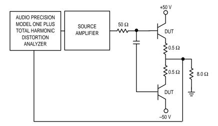
Figure 17. Total Harmonic Distortion Test Circuit
