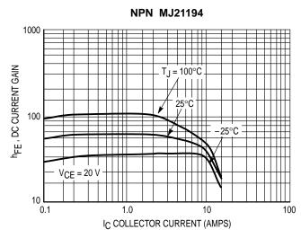
Figure 6. DC Current Gain, VCE = 5 V
