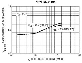
Figure 12. Typical Base-Emitter Voltage
