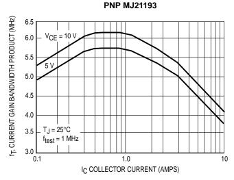
Figure 1. Typical Current Gain Bandwidth Product
