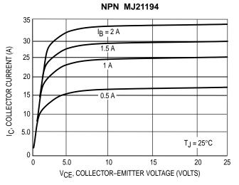
**Figure 8. Typical Output Characteristics**
