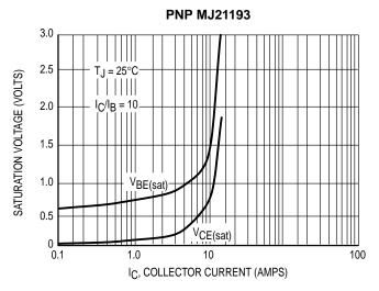
Figure 9. Typical Saturation Voltages
