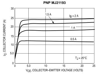
Figure 7. Typical Output Characteristics
