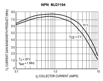
Figure 2. Typical Current Gain Bandwidth Product
