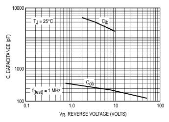
Figure 14. MJ21193 Typical Capacitance
