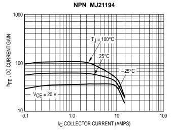
Figure 4. DC Current Gain, V<sub>CE</sub> = 20 V
