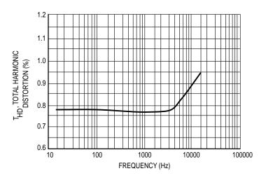
Figure 16. Typical Total Harmonic Distortion
